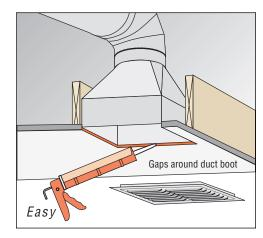
One rule is that if you are in the attic and can see the back side of an interior wall, you should seal and insulate over that chase. Some penetrations, such as duct boots, can be sealed from the living space side.
