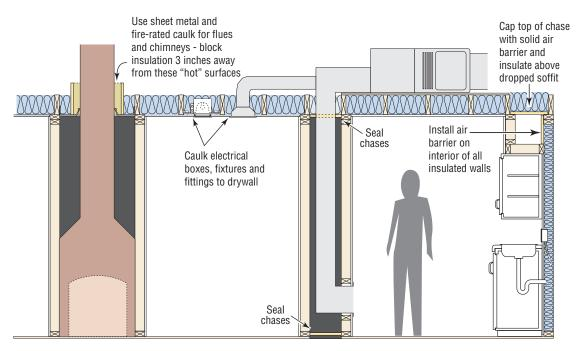
Some chases extend from attic to basement or crawlspace - block and seal both ends.
