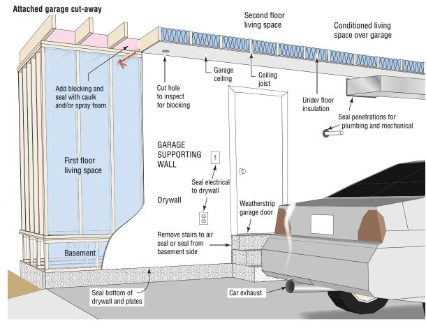
Air sealing garage penetrations can present a challenge. Easy tasks involve caulking obvious penetrations such as electrical outlets, the drywall perimeter and bottom plates of the foundation. More difficult tasks involve cutting away ceiling drywall in the garage to check for and provide blocking between the garage and the floor system adjacent to the garage.
