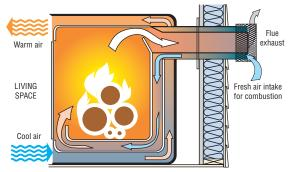
A sealed combustion fireplace provides fresh air for combustion. A heat-exchanging chamber around the firebox improves the efficiency.
