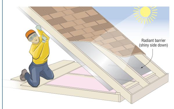
Use walkboards as walking surfaces. If working on the roof, always have someone close by in case of an accident. Work during a cool part of the day, as roof temperatures can exceed 150 degrees on hot, sunny days.
