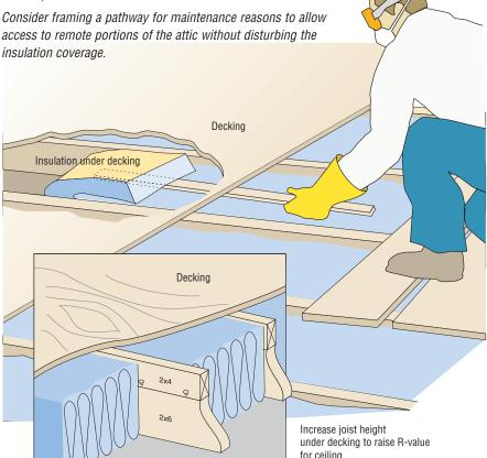
Installing insulation under existing attic decking requires some improvising to avoid removing the decking. Be sure to wear proper protective gear and clothing when installing any insulation. Install batt insulation with the vapor barrier down in attics with no insulation. If adding insulation on top of existing insulation, use batts without a vapor barrier backing or remove the backing.
