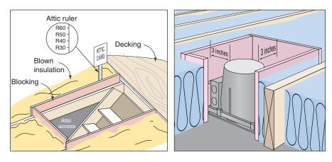
Attic rulers are required for loose-fill insulation and are a helpful guide to ensure adequate coverage. Create dams to hold back insulation and to maintain levels. Attic access such as scuttles and drop-down stairs benefit from a insulated cover.
