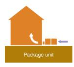
A **packaged system** has the air conditioner and furnace or the heat pump components contained in one larger outdoor metal box. There is one large supply and return duct connection from the outdoor equipment to the home's duct system.
