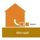
installed as wall-mounted ductless units (although short ducted runs are possible), and offer potential for zoning. They are ideal for conditioning additions and smaller zones such as bonus rooms. Ductless mini-splits usually heat and cool a room or two while ducted models can provide comfort to an entire home. Certain manufacturers offer variable speed and capacity units which can result
