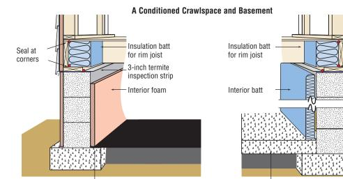
6 mil polyethylene and laps up foundation wall 6 inches
