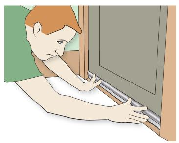
**Older doors and windows** are more difficult to airseal. Most have single pane windows held in place with putty and insuring they are properly secured is the first step. There are various types of weatherizing and airsealing materials that can be creatively used including adhesive backed foam, metal or plastic v-seal, rubber bulb type, etc...
