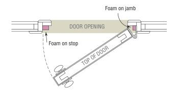
If **doors** are not warped, adhesive-backed foam on the door stop is easiest. Install on the hinge side of the door jamb (door frame side where the hinges are mounted), not on the door stop in order to prevent the foam from being pinched when the door closes.
